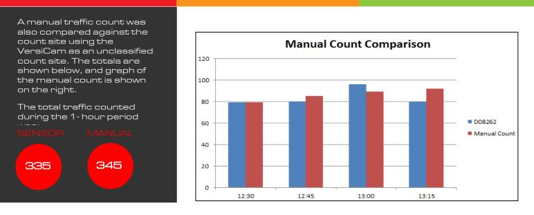
This shows that the manual counts, and the SCOOT detector's automated counts were very close. The differences can be explained as follows:
